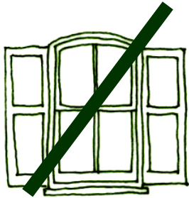
The 2-panel shutters do not fit the arched opening Not Recommended
